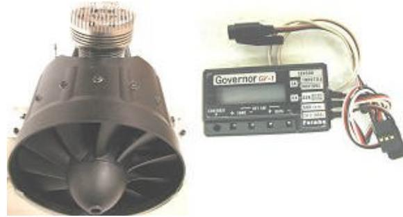
Figure 09 –Ducted Fan Unit & GV1 Flight Governor
