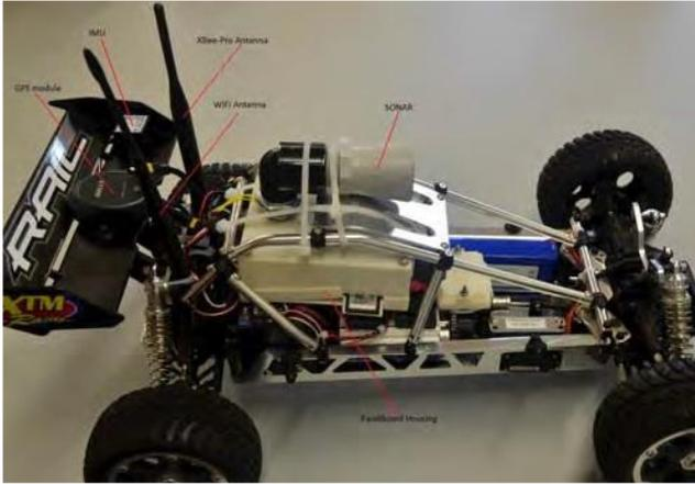
Figure 4. UGV Modified RC XTM Rail
