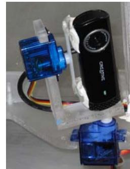
Figure 6. Web camera mounted sideways.
