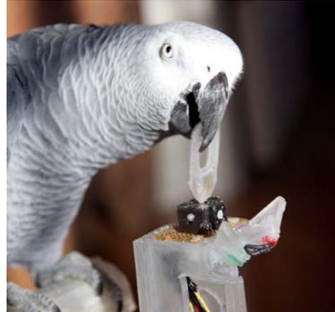
**Figure 8. Polycarbonate joystick activated by the bird.**
