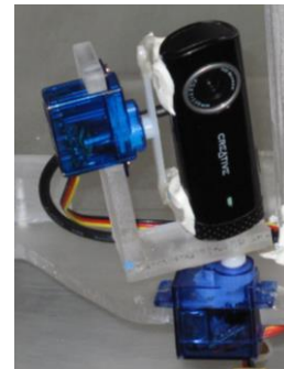
Figure 6. Web camera mounted sideways.
