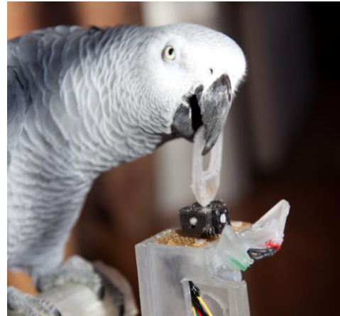
Figure 8. Polycarbonate joystick activated by the bird.
