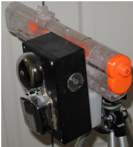
Figure 1. Sound activated squirt gun.
