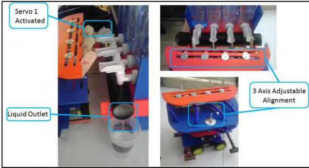
Figure 6. Cam alignment and adjustability
