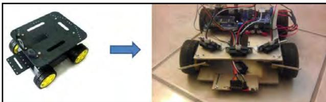
Figure 14. DFRobot chassis and early DriMix 4ics model
