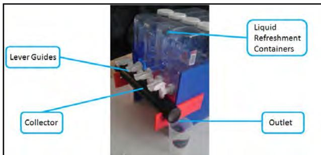
Figure 3. Mixing station principle components
