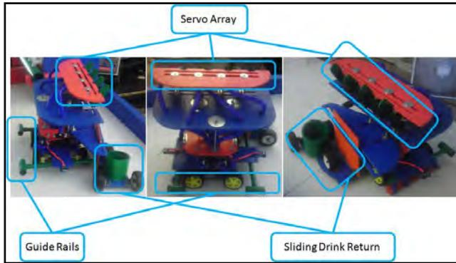
Figure 2. Mobile platform principle components
