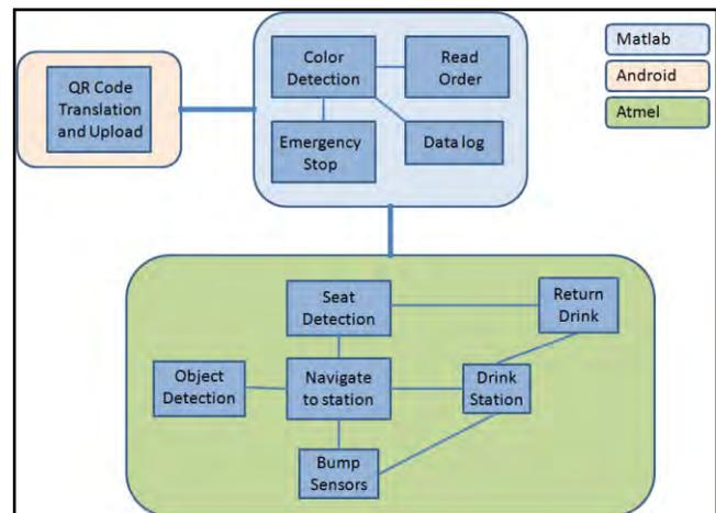
Figure 1. DriMix 4ics systems block diagram
