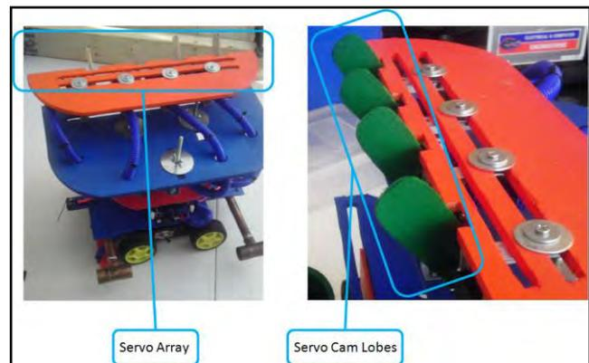
Figure 5. Servo array and cam lobes
