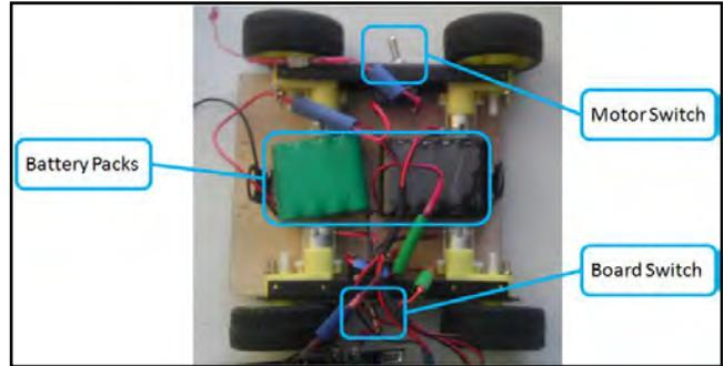
Figure 12. Battery packs and power switches
