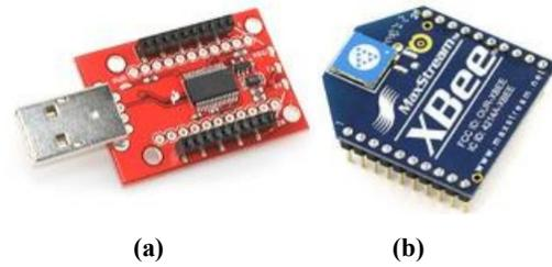
Figure 13. (a) Xbee Explorer USB dongle; (b) Xbee wireless RF chip
