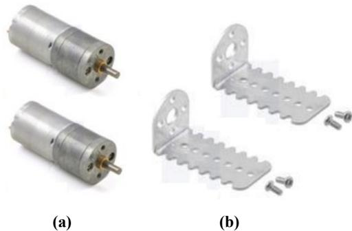
**Figure 7. (a) 75:1 metal gearmotors, 75 RPM, 80mA free-run, 2.2A stall, 85 oz-in (6.1 kg-cm); (b) 25D mm metal gearmotor brackets**
