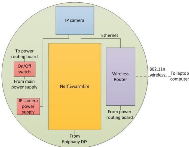
**Figure 4. MARS platform top piece layout**
