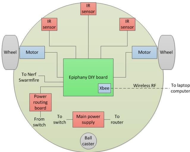
**Figure 3. MARS platform bottom piece layout**
