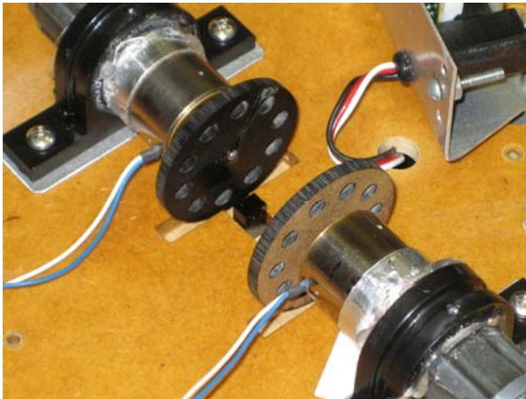
Figure 4. Code wheels attached to the motors.
