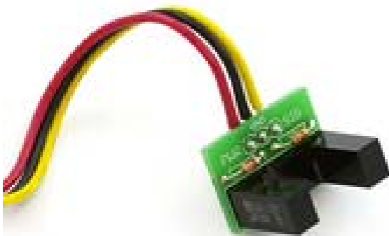
Figure 3. Sparkfun photo interrupter [2]
