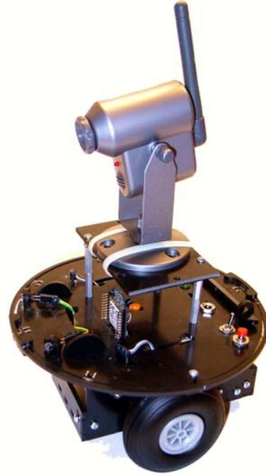
Figure 1: TJ Pro-Avr™ robot vision system.
