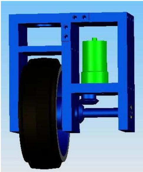
Figure 6. Solid model CAD of Gnuman's wheel assembly.
