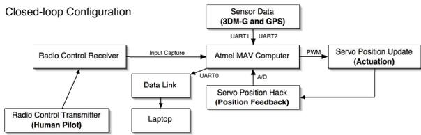
Fig. 2. Block Diagram of On-board Hardware
