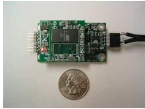
Fig. 3. MAV Atmel-based Computer - MAV128
