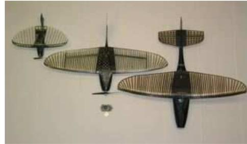
Fig. 1. MAV Platforms: 10", 24", and High Capacity 24"
