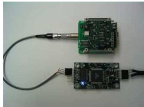
Fig. 4. MAV128 Computer with 3DM-G
