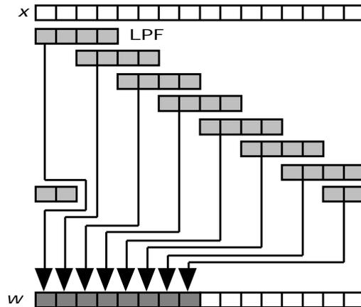
Figure 3: First step in computing the 1-d wavelet transform: low pass filtering (in increments of two) on an input signal  $x$ .
