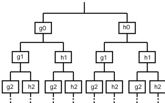
Figure 6: “Balanced” tree for wavelet decomposition.
