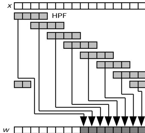
Figure 4: Second step in computing the 1-d wavelet transform: high pass filtering (in increments of two) on an input signal  $x$ .
