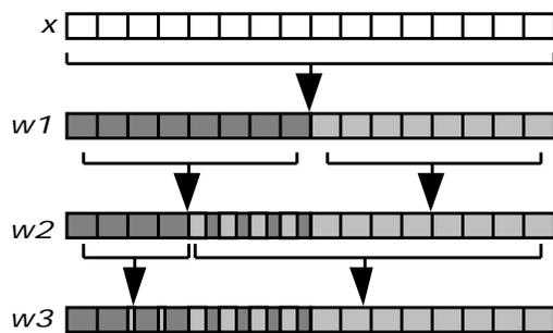
Figure 5: Three level wavelet transform
