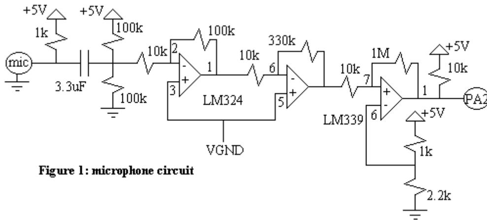
**Figure 1: microphone circuit**
