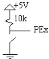
**Figure 2: contact switch ckt**
