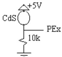
**Figure 3: CdS circuit**
