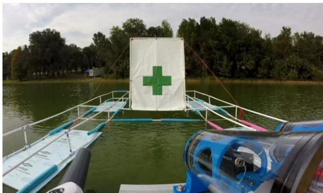
Fig 13. The Identify Symbols and Dock platform that was constructed to aid in the field testing of NaviGator ASV
