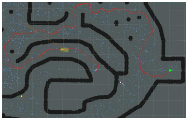
Fig 7. The NaviGator ASV's real-time ROS-integrated RRT algorithm being run on an arbitrarily drawn, complicated occupancy grid
