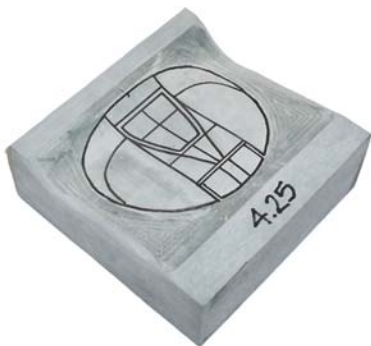
Figure 7. Completed wing tool ready for composite lay up process
