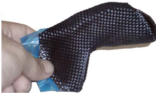
Figure 9. Fuselage laid up on tool
