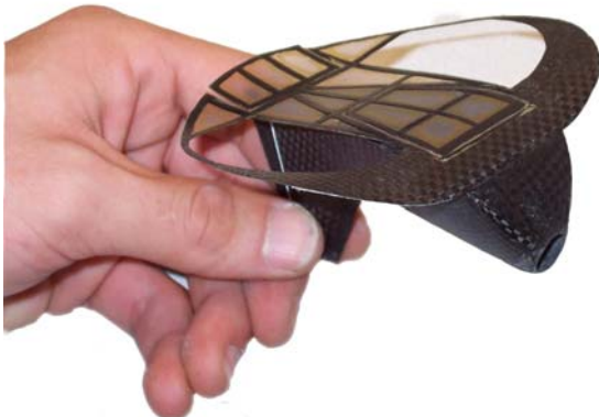
Figure 10. Wing and fuselage joined with CA
