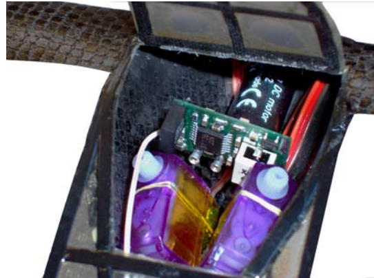
Figure 11. Servos installed in fuselage with motor and radio
