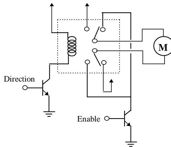
**Figure 1. Motor driver schematic**
