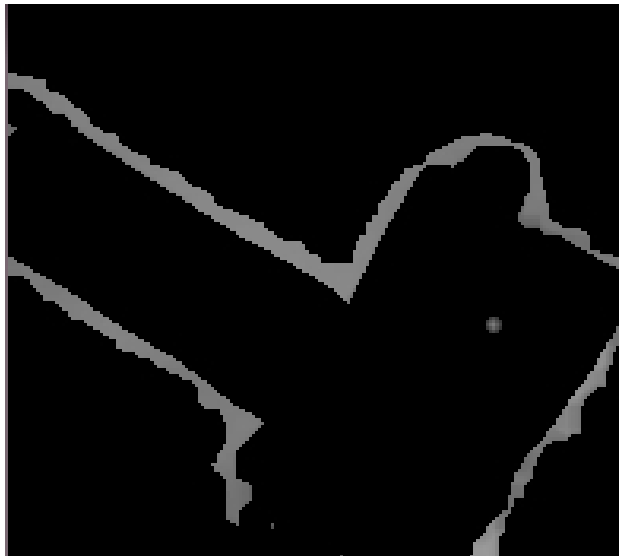
Figure 8. Processed image showing landing dock border and circular target
